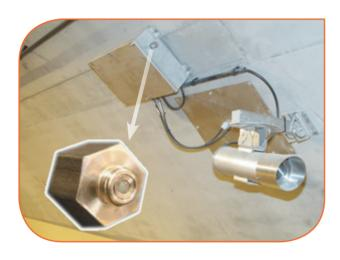
Special microphones were developed which are able to withstand the rough conditions in tunnels. The microphones were subjected to comprehensive splashing water and ageing tests, the results of which were validated by acoustic measurements.
